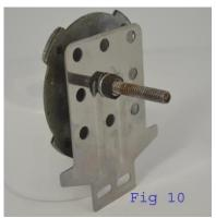
In this case the stud fit through the ¼ inch hold in the adaptor plate. If it hadn't the hole can easily be opened to the appropriate size with a drill. In Figure 10 there is a nut on both sides of the adaptor plate. This allows the badge to be moved in and out to match the depth of the other badges. A lock washer between the nut and adaptor lets you lock it in place.
