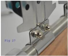
While the finish hardware is still snug you can move the clip left and right to get the spacing right. The spacing will depend on the size and shape of the badge itself. When you are satisfied with the arrangement tighten the hardware to keep everything in place. The hardware only needs to be tight enough to keep the badge from falling over.
